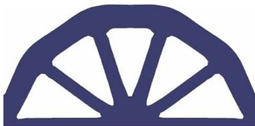
**Fig. 12** Optimization result of the Michell type structure without the geometric constraint [36]
