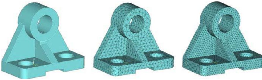
Figure 13. Pedestal body for computing natural frequencies and model
