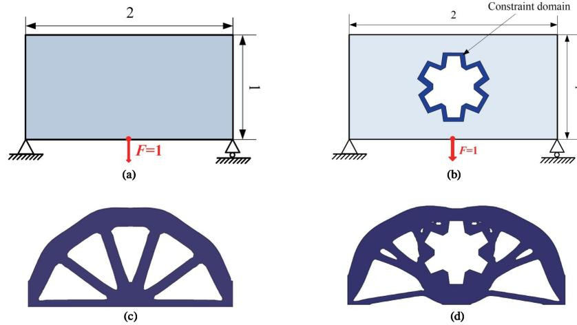
**Figure 12:** The level-set-based ITO of the Michell type structures: (a) Design domain without geometric constraint, (b) Design domain with geometric constraint, (c) Optimization result without geometric constraint and (d) Optimization result with geometric constraint [Wang and Benson (2016b,a)]
