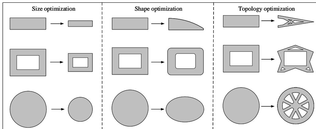
**Figure 1:** An illustration of structural optimization
