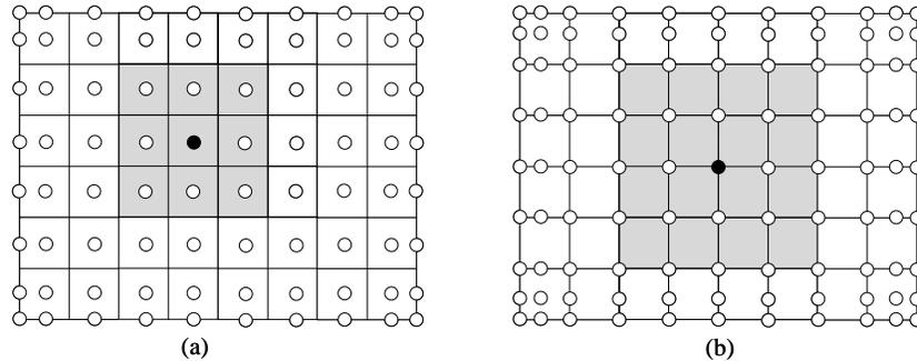
**Figure 7:** An illustration of the B-spline basis support region corresponding to the black solid control point: (a)  $p = q = 2$  and (b)  $p = q = 3$
