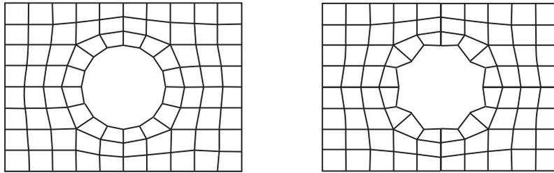
**Figure 3:** Schematic of jagged boundaries occurring during a shape optimization for a FEM-based shape optimization
