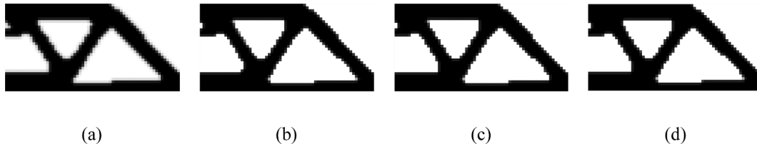
Fig. 20. The final optimized structures of CITO (a) and local-update ITO with different \rho_s : (b) \rho_s = 0.1 , (c) \rho_s = 0.2 , (d) \rho_s = 0.3 .
