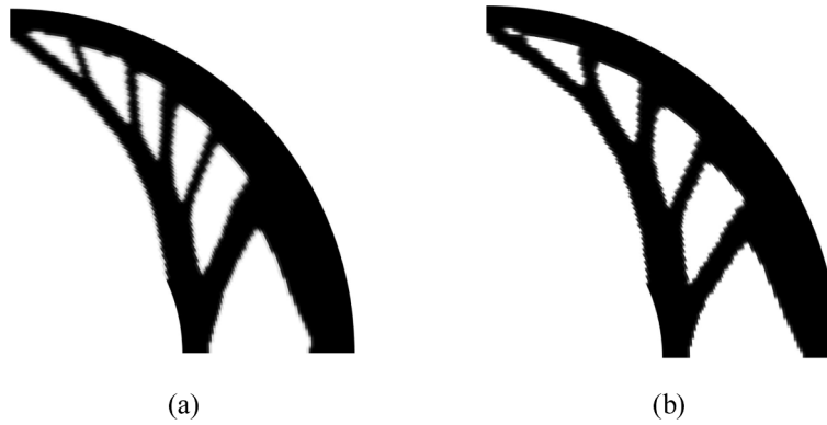
Fig. 24. The final structure of quarter annulus with (a) CITO and (b) HITO.
